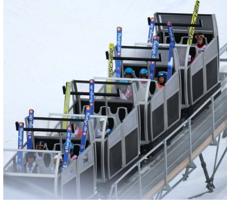
The new uphill and downhill cableway for the Adlerschanze ski jumping hill in Hinterzarten is a modern pull-rope solution by Wiegand allowing up to 24 passengers to climb a height difference of 80 metres at a speed of up to 2.4 m/s. (Image: Wiegand)
